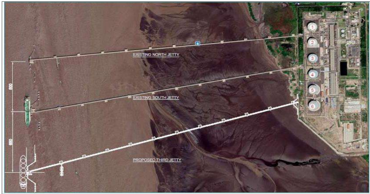
Figure 2.2: Location of Proposed third berth (jetty)
